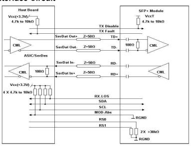
TD-/+: These are the differential transmitter inputs. They are AC-coupled, differential lines with 100Ω differential termination inside the module. The AC coupling is done inside the module and is thus not required on the host board. The inputs will accept differential swings of 150 – 1200 mV (75 – 600mV single-ended).
